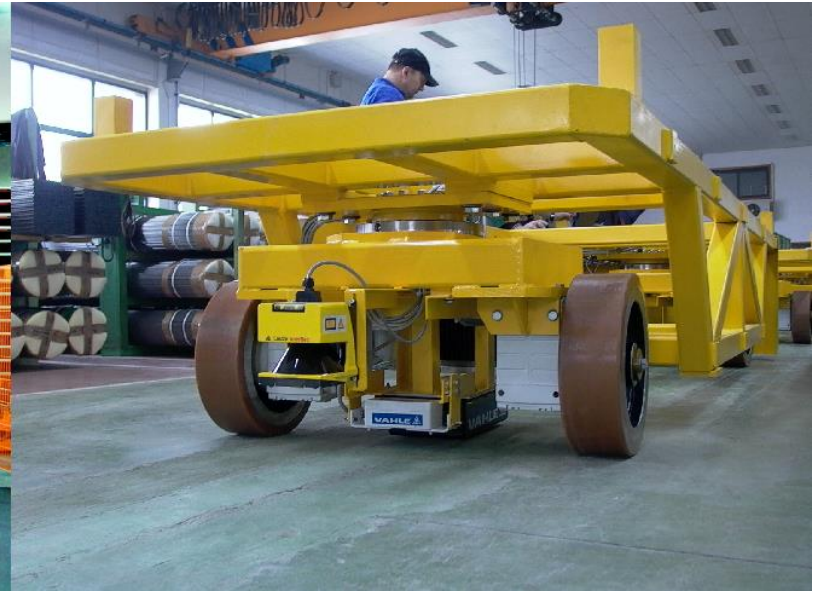
1.5 kW AGV-supply with track guiding sensor in Tubos del Mas / Spain
