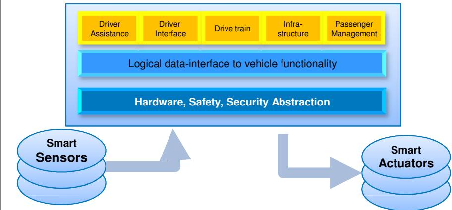
**Platform must provide ASIL-D with fail-operational behavior**
