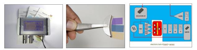
CO<sub>2</sub> system (left), CO<sub>2</sub> sensitive layer (middle), evaluation kit (right)
