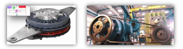
The Smart Sensor and Clutch-brake unit (left) for industrial equipment (right)
